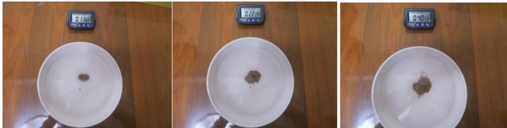
Figure 8: Dispersive test on the sample ( depth- 4ft) from Sangling Church, Hakha, GPS Point: (0563476 E, 2504958 N)
