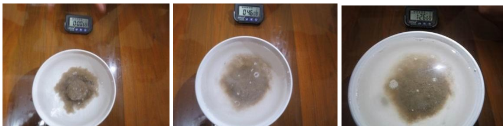
Figure 9: Dispersive test on the sample (depth- 12ft) from Sangling Church, Hakha GPS Point: (0563476 E, 2504958 N)
